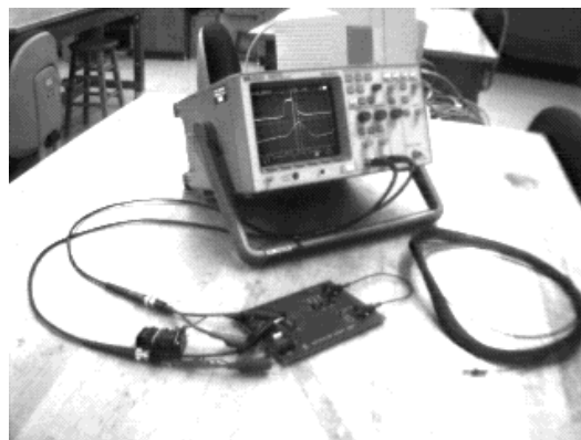
Figure 5: A set up similar to this was used to measure the speed of light [5]
