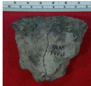
Figure 17 TAM 940.3 This crucible was used for smelting. We can make this assumption because of the slag deposits found on the interior and exterior surfaces of the artifact.
