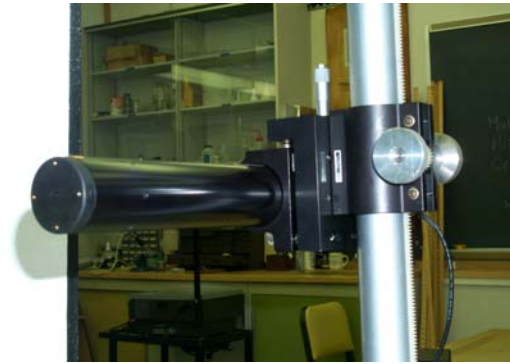
Fig. 8: Helium-Neon laser used for the experiments
