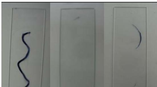
Figure 6. Results of wiping on the (left to right) control, OPA, WD-40 slides without an ethanol
