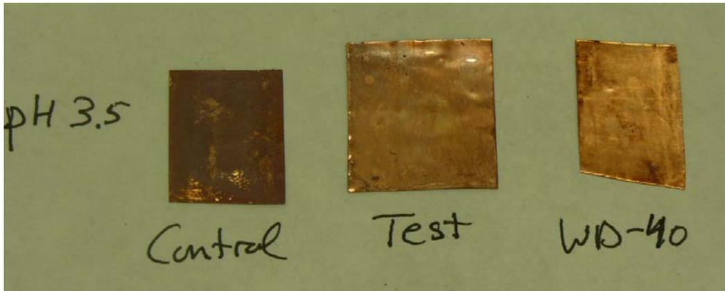
Control, OPA-layered, and WD-40<sup>®</sup> applied copper samples in solution of pH 3.5
