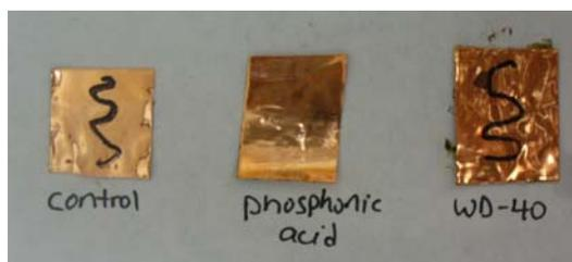
Figure 9. The copper surfaces are shown with applied Sharpie<sup>®</sup> ink after the wipe test.
