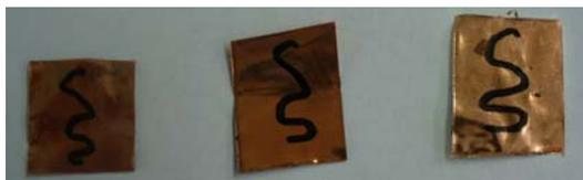
Figure 8. The copper surfaces with applied Sharpie<sup>®</sup> ink before the wipe test
