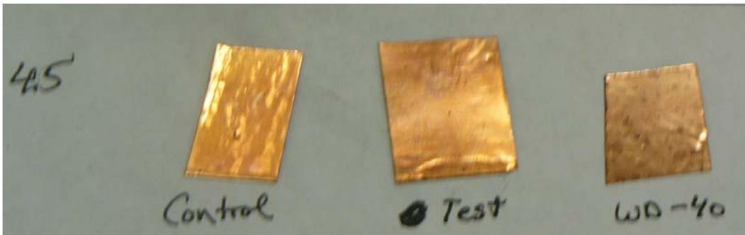
Control, OPA-layered, and WD-40<sup>®</sup> applied copper samples in solution of pH 4.5
