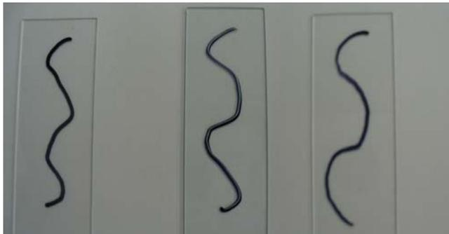
[From left to right] Control, OPA, WD-40<sup>®</sup> glass slides with applied Sharpie<sup>®</sup> ink before wiping
