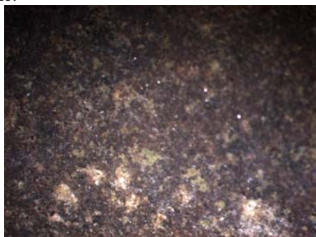
Figure 8N: Magnification 5x. Side after grinding leaves against stone. Slightly increased amount of pitting visible.
