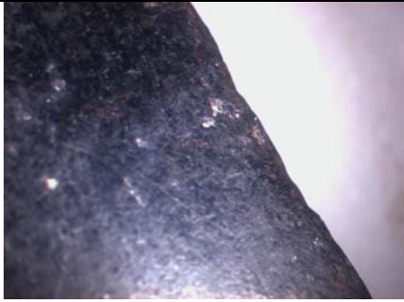
Figure 8E: Magnification 10x. Notches perpendicular to the blade, white pits, and slight red-brown discoloration visible. Blade is dull.
