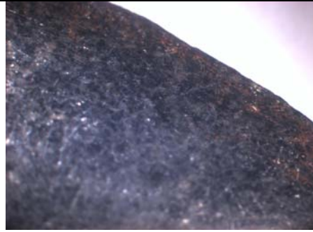
Figure 8F: Magnification 10x. Red-brown discoloration along edge and some notches perpendicular to the blade visible. Blade is dull.
