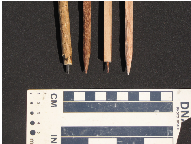
Figure 6: From left to right, chert microdrill, teak, copper, and red oak drill shafts
