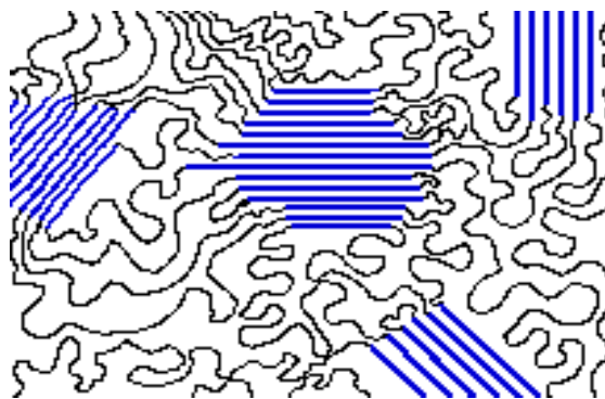
Figure 3. Crystalline (blue) and amorphous regions in a polymer. Amorphous regions allow for a greater rate of diffusion (3).
