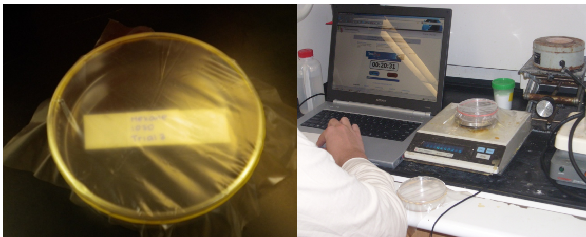
Figure 7. Apparatus. This shows a petri dish covered with a polymer membrane (left) as well as a scale and stopwatch used to take mass and time measurements.
