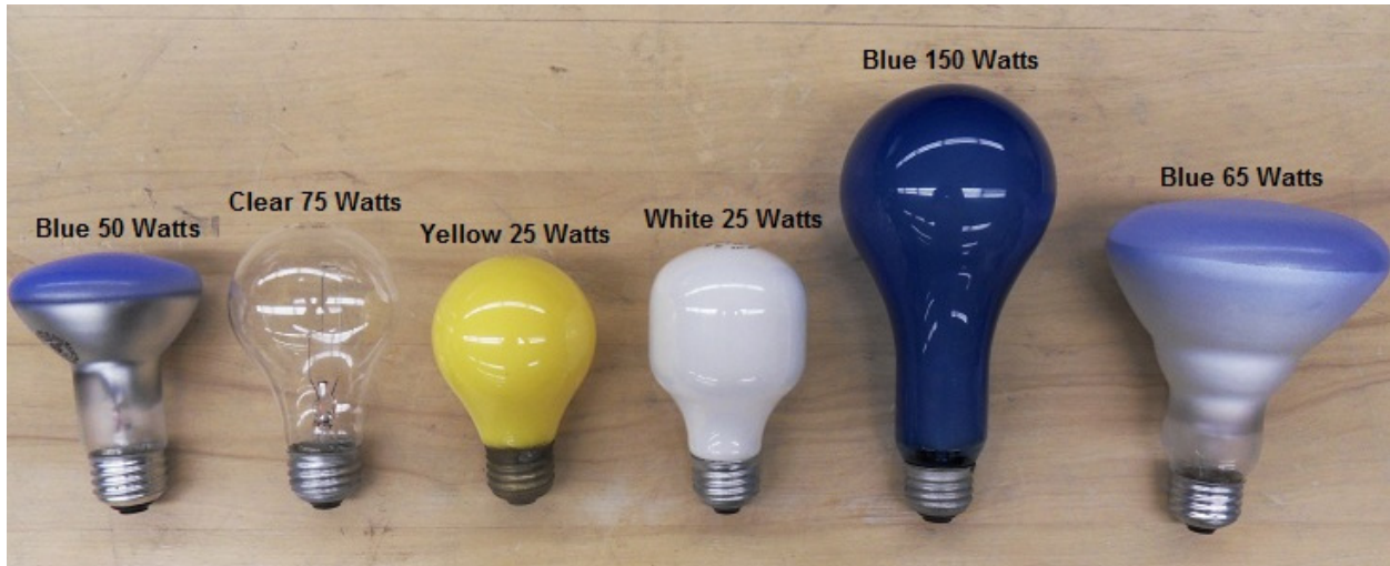
Figure 2 The six types of light bulbs used to test each solar cell.
